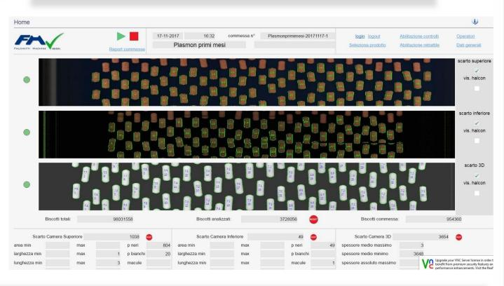
FM VISION has developed and implemented a fully automated system for complete control of cookies or similar directly on the transport conveyor, with speeds up to 200pz / sec
